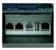
Secure Connector Panel A combination of 3 Serial, 1 USB and 1 Ethernet port are hidden behind a convenient, easy to access door located on the back of the unit.
